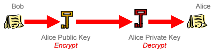
Figure 3.1.2.1 Asymmetric Cipher Process
